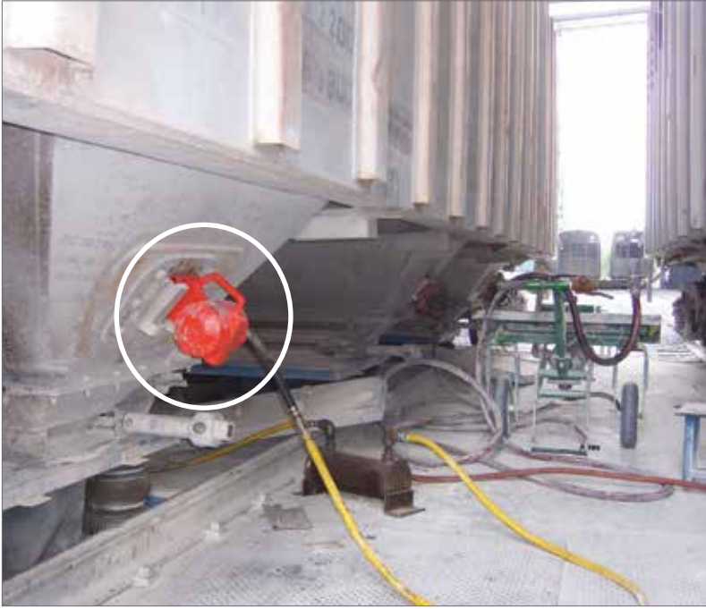
Above: A Series SVRWS-5500 (page 58-59) railroad car shaker on the job.
