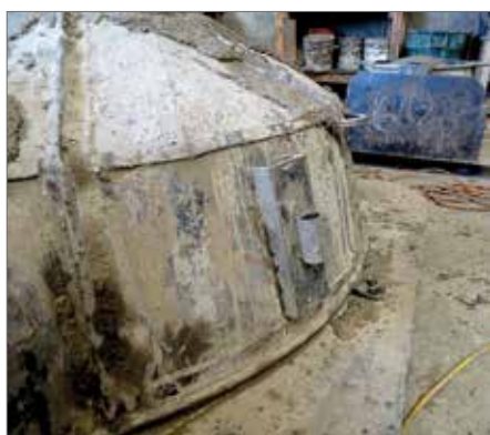
UPF bracket is ideal for precast and other applications. Vibrators can be easily moved.
