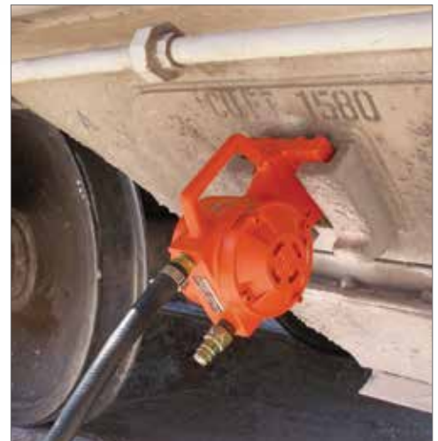
The CCW-5000 unit shown here fits the standard rail car female wedge bracket for easy unloading of a rail road hopper car.
