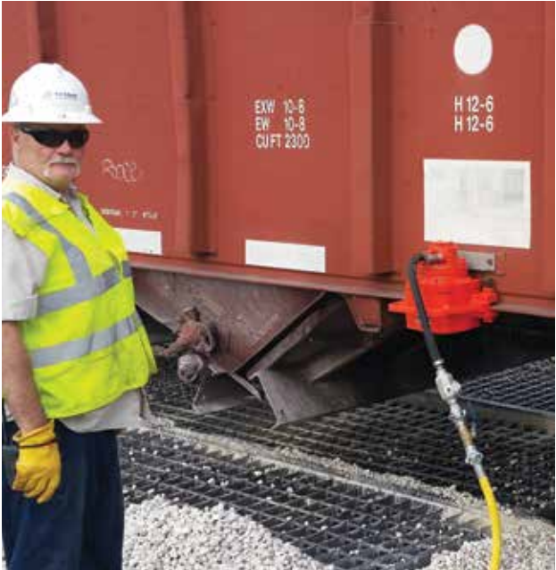
Above: A PC-3500 Big Buster (see page 34-35 and 58-59) shakes a railroad hopper car with it's high force and low frequency. It easily clamps to the railcar and can be moved from place to place.
