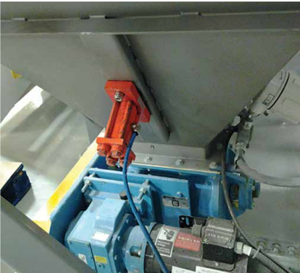
Above: Mounting this 50-2 unit (as seen on page 24) on a hopper will help to dispense a better quality product with accurately measured material for more consistent batches. It will also lead to a more efficient and standardized process with predictable scale weights. No more labor time wasted banging on the hopper walls to release stuck material.
