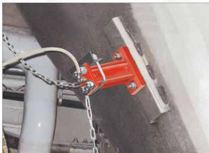
The LI Piston is used when an adjustable impact is desired to break up material bridges or ratholes.
