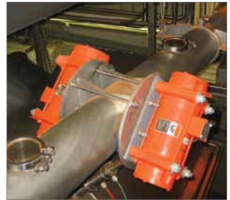
Consistent material flow is maintained by dual units in this pipe line.
