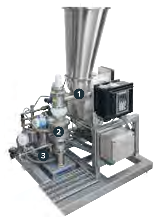
Continuous inline dispersion set-up: 1. Continuous feeder, 2. Uniform film interface (UFI) 3. ZC Powder Dispenser.
