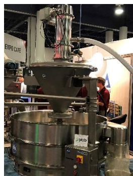
piFLOW P Filling a SWECO
